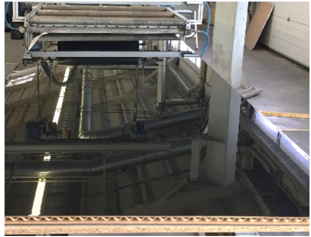
Coating with roll goods at the calender press
